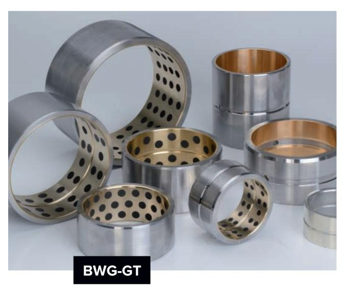
BWG-GT bearings with or without flange are made of casted bronze material with a steel shell and special solid lubricant embedded.
